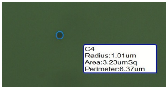
FIG. 9. Photograph of CR-39 at 40\times magnification. A very small track oriented on the back side of the SSNTD indicates the presence of a proton. This location requires the particles detected to be considerably more energetic to traverse through the entire 200\mu\text{m} thick detector.
